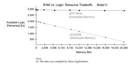
In addition, XC4000E devices require built-in synchronization circuitry for every 16 bits of RAM. Consequently, implementing a 2-Kbit block of RAM requires 128 copies of the same synchronization circuit. Additionally, when a CLB is used for logic, the memory write synchronization circuitry still exists in silicon, even though it serves no purpose. For the same 2 Kbits of RAM, FLEX 10K devices require only a single synchronization circuit.
